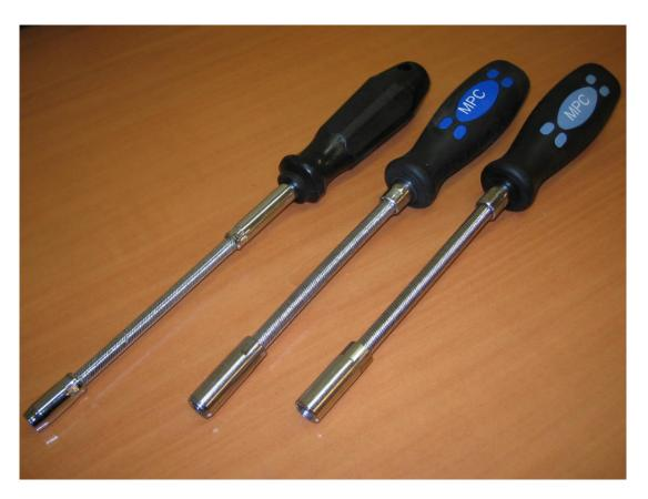
Flexible sockethead screwdrivers for easy mounting of wormdrive clamps.
